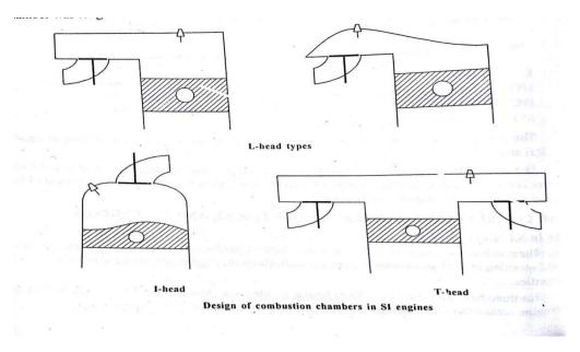
Side valve engine was introduced in petrol engines, in 1910 - 30. In this type valves are placed side by side. It is easy to lubricate the valve mechanism. It had the defects like lack of turbulence, extremely prone to detonation, slow combustion process etc.
