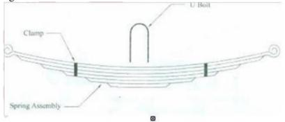
Fig: Semi elliptical leaf spring
