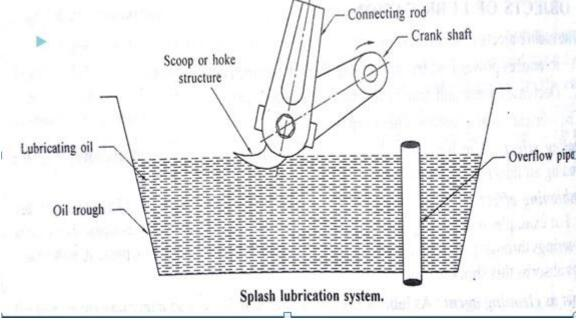
Fig: Splash lubrication system
