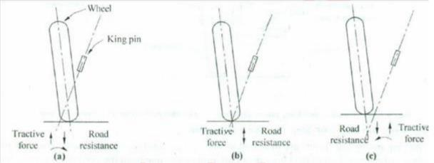
Fig: The wheel and king pin centre line meet (a) above the ground (negative scrub radius) - wheels toe in (b) Exactly on the ground (zero scrub radius - 0 effect and (c) below the ground (positive scrub radius) - wheels toe out
