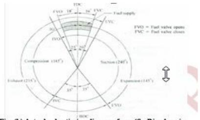
Fig: (b) Actual valve timing diagram for a 4S - Diesel engine
