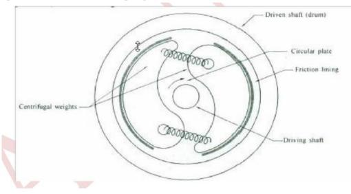
Fig. Centrifugal Clutch
