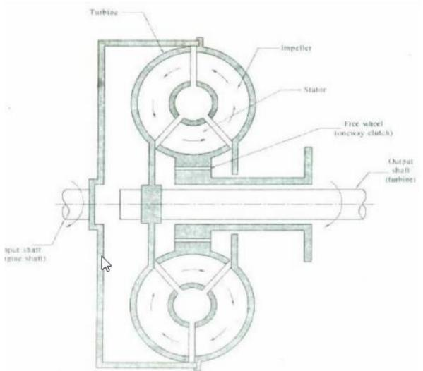
Imagine you have two fans facing each other. Turn one fan on, and it will blow air over the blades of the second fan, causing it to spin. But if you hold the second fan still, the first fan will keep right on spinning.
