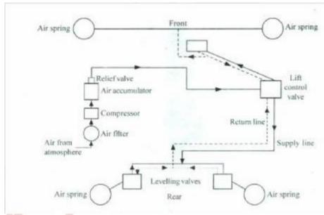
Fig: Layout of air suspension system
