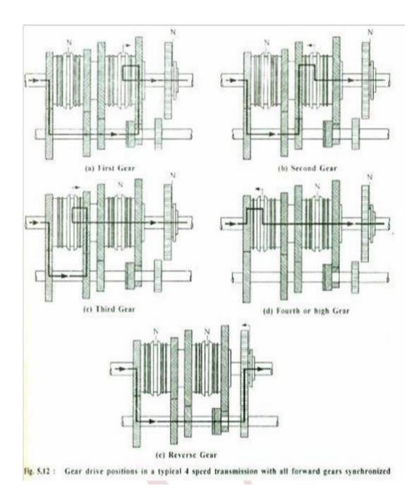
Gear teeth are helical cut, with the exception of the reverse sliding gear and rear reverse idler gear. Figure (a) to (e) shows gear drive positions for various speeds.
