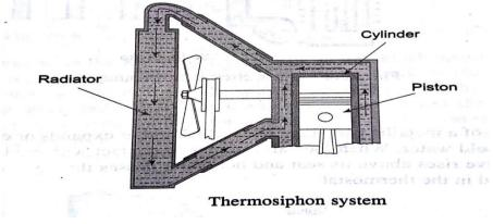
Fig (a): Thermosyphon Cooling System
