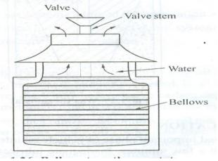
**Fig. Bellows type thermostats**
