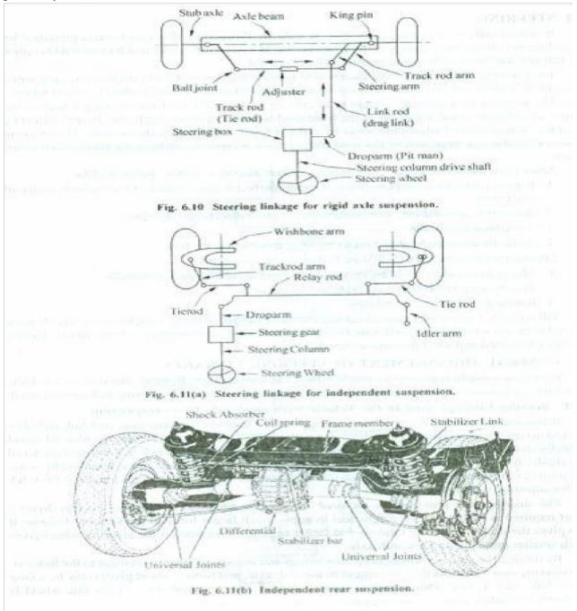
Steering Linkage used for Independent front suspension
