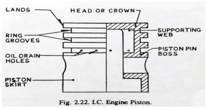
Fig: Typical I.C, engine piston
