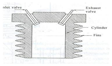
Fig. Cylinder with Fins
