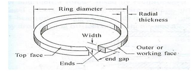
The material generally used for piston rings is fine grained alloy cast iron containing silicon and manganese. It has good heat resisting qualities. Rings with molybdenum filled face have also been introduced recently. Alloy steels are also used. The number of rings vary depending on the engine design. It varies from two to four.
