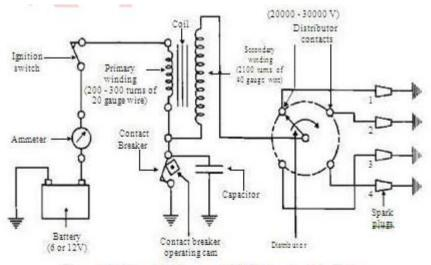
Figure 4,2.; Schematic Diagram of Coil/Battery Ignition System
