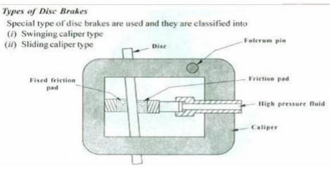
Fig: Disc brake of swinging caliper type
