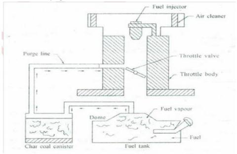
Fig: ECS for an engine with throttle body injection
