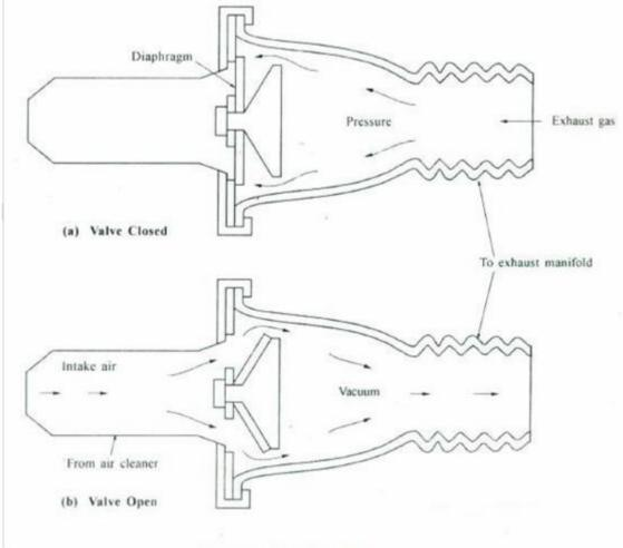
The air aspirator valve closes when exhaust valve opens which causes pressure in the exhaust manifold to increase above atmospheric.
