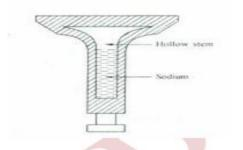
Fig: (b) Sodium Cooled Valve
