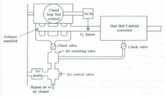
Fig: Air Injection System
