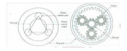
Simplified view of planetary gear system (b) Planetary gear system
