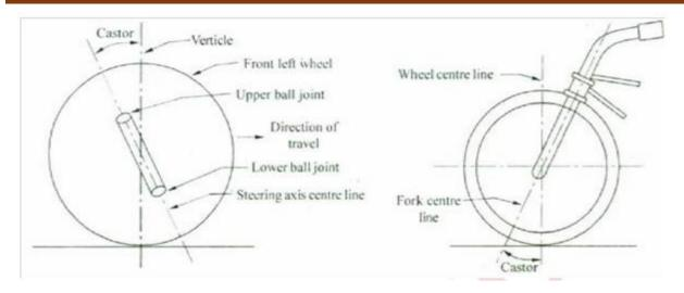
Fig: (a) Castor; (b) Castor on front wheel of the bicycle.
