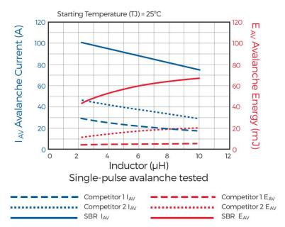
*Figure 5. The SBR's superior avalanche ruggedness compared to Schottky diodes allows the use of lower-rated devices for greater efficiency.*
