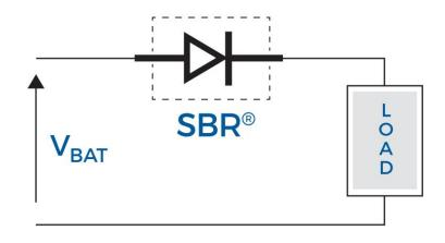
Figure 2. The SBR is connected in the same way as a diode or MOSFET, with no charge-pump circuitry required.
