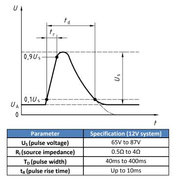
*Figure 6. Knowing the device's surge-current capability helps determine ISO 7637 Pulse 5a survivability.*
