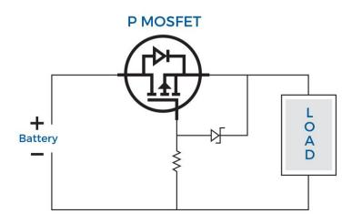
Figure 1b: A P-channel MOSFET used for reverse-battery protection device requires fewer components but incurs higher power losses
