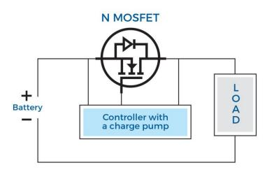
Figure 1a. The charge pump needed to supply the MOSFET gate voltage increases complexity and may introduce EMI issues.
