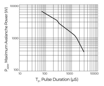
Figure 4: Pulse duration versus maximum avalanche power (for Diodes Incorporated's SBR30A60CTBQ device)
