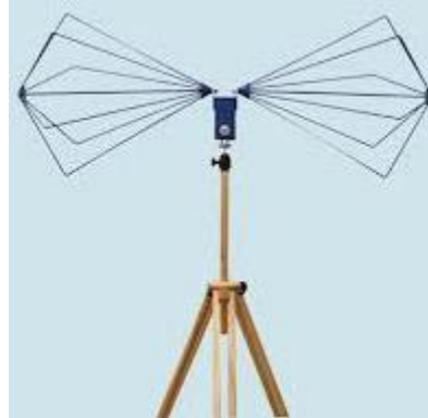
Biconical Antenna: 30 to 300 MHz
