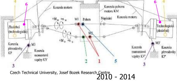
Strain-gauge flange for constant torque measurements
