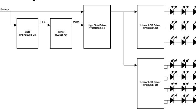
Figure 1. TIDA-00846 System Block Diagram
