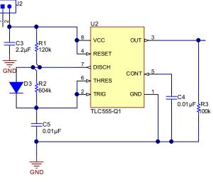
Figure 4. PWM Circuit
