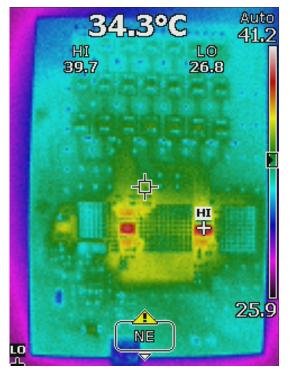
Figure 10. Thermal Image of Tail Function at 25°C, 12-V Input Voltage
