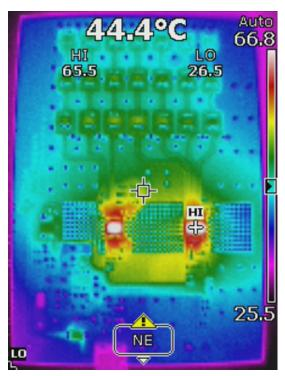
Figure 9. Thermal Image of Stop Function at 25°C, 12-V Input Voltage
