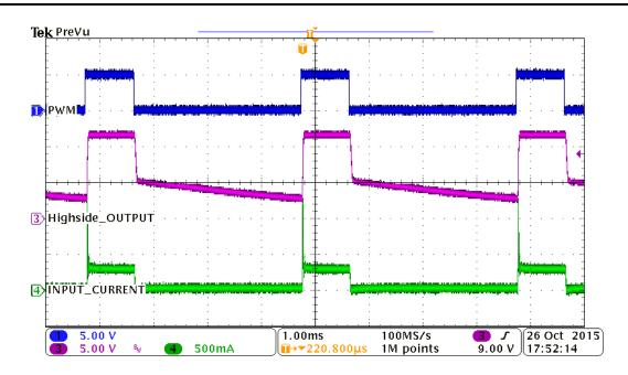
Figure 6. Tail Function Waveform—20% PWM Duty Cycle Input Voltage and Current
