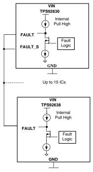
Figure 2. Fault Bus of TPS92630-Q1 and TPS92638-Q1
