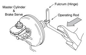
Fig. 7.3 Brake pedal – pendant type lever (Example 7.3)
