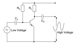
Fig. 18.10 Voltage amplifier
