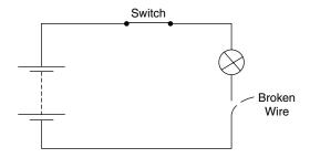
Fig. 17.11 Open circuit
