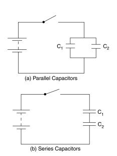
Fig. 17.32 Capacitors in circuits
