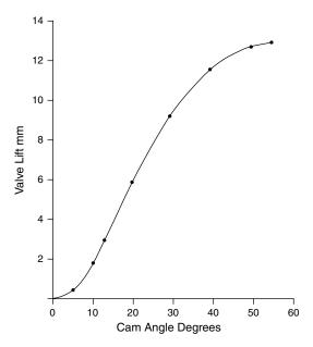
Fig. 3.4 Valve lift and cam angle (Example 3.24)
