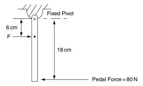
**Fig. 7.4** Simple lever equivalent of brake pedal (Example 7.3)
