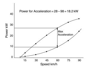
Fig. 11.5 Graph of power vs. speed (Example 11.3)
