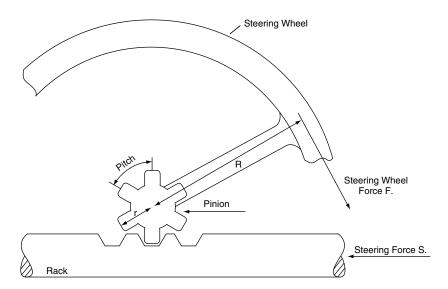
Fig. 8.7 Rack and pinion as a machine
