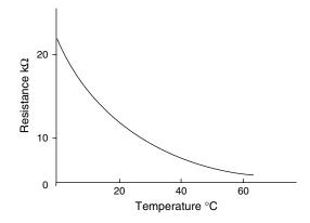
Fig. 17.14 Negative temperature coefficient
