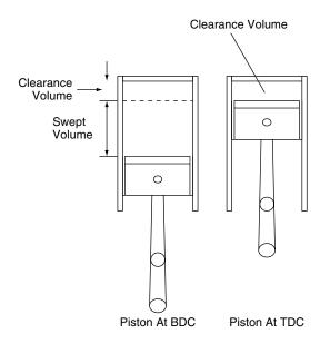
Fig. 1.3 Compression ratio (Example 1.29)
