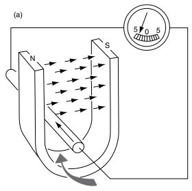
An EMF (Electromotive Force) is Produced in the Wire Whenever it Moves Across the Lines of Magnetic Flux.
