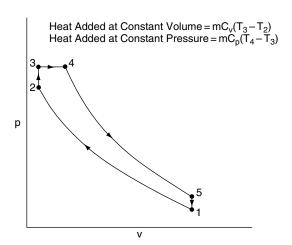
Fig. 15.4 pV diagram for the dual combustion cycle
