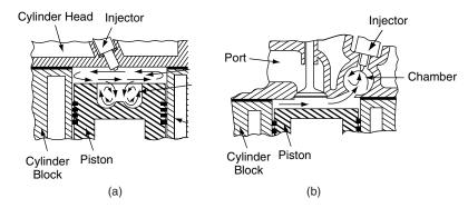
Fig. 16.2 Direct and indirect injection
