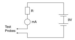
Fig. 17.10 Principle of the ohmmeter
