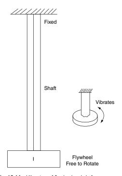
Fig. 12.16 Vibration of flywheel and shaft
