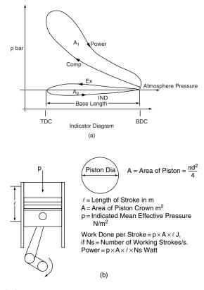
Fig. 14.4 Indicated power calculation
