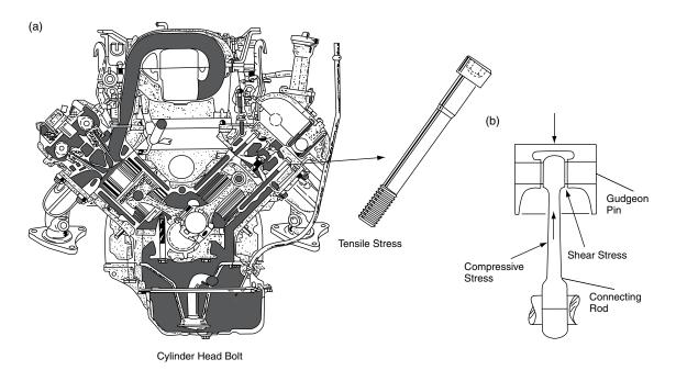
Fig. 6.2 Components under stress
