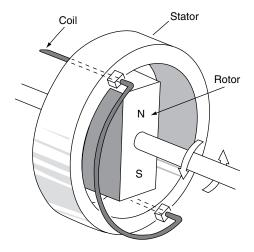
Fig. 17.25 The vehicle alternator
