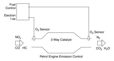
Fig. 16.6 A 3-way catalyst emission control system
