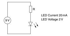
Fig. 18.7 The current-limiting resistor - LED
