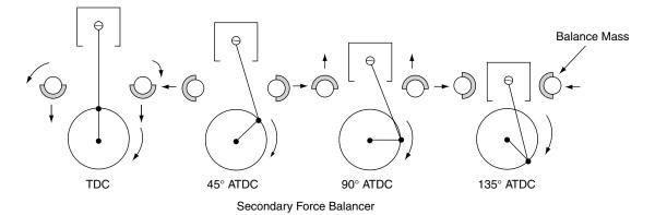
Fig. 12.10 Secondary force balancer
