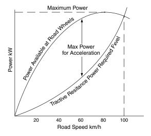
Fig. 11.4 Graph of power required vs. power available
