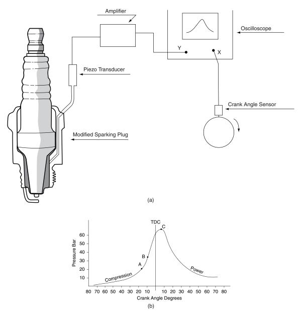
Fig. 14.5 (a) A high-speed engine indicator; (b) cylinder pressure vs. crank angle
