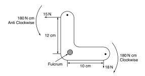
Fig. 7.5 A bell crank lever
