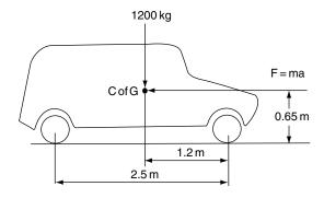
Fig. 11.2 Calculation of load (Example 11.1)
