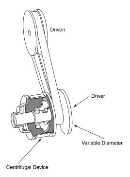
Fig. 9.17 Belt drive variable ratio
