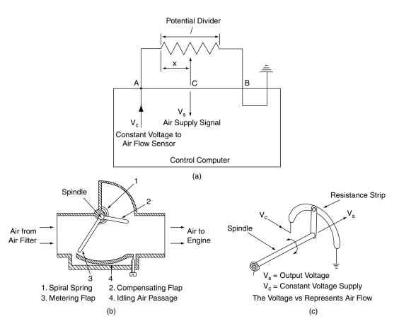
Fig. 18.16 Air flow sensor
