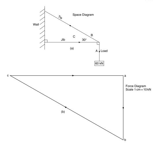
Fig. 5.6 Triangle of forces (Example 5.2)
