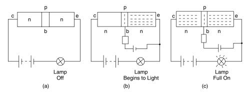
Fig. 18.8 A simple transistor
