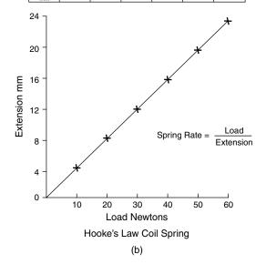
Fig. 5.11 Hooke's law apparatus and results
