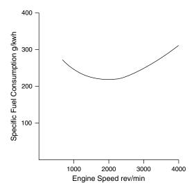
Fig. 14.9 Specific fuel consumption vs. engine speed
