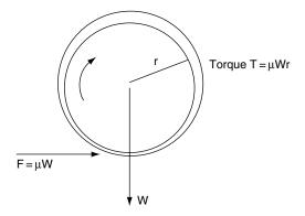
Fig. 9.16 Friction in a journal bearing
