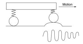
Fig. 12.17 Undamped free vibrations of vehicle suspension
