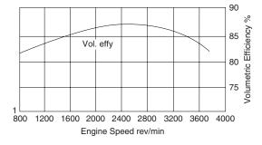
Fig. 14.7 Volumetric efficiency - diesel engine
