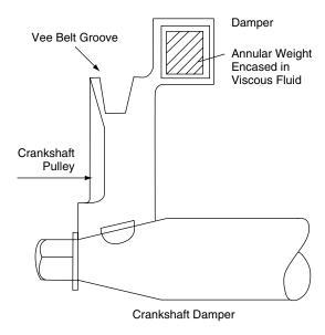
Fig. 12.19 Crankshaft vibration damper
