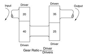
Fig. 1.2 Gearbox ratio (Example 1.27)
