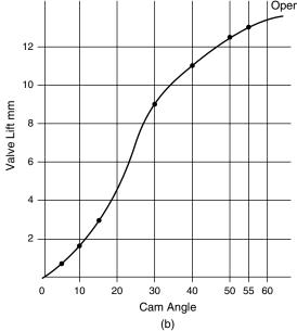
Fig. 12.20 Valve lift
