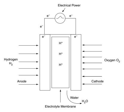
Fig. 16.8 A simple fuel cell
