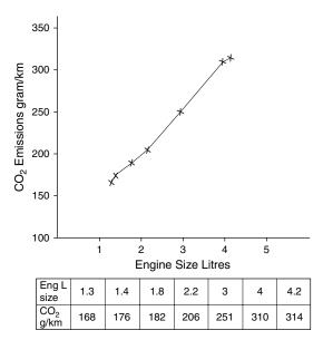
Fig. 3.2 Graph of carbon dioxide emissions (Example 3.22)
