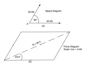
Fig. 5.5 Parallelogram of forces (Example 5.5)
