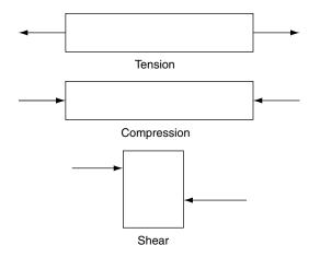
Fig. 6.1 The three basic stresses
