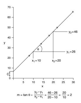
**Fig. 3.5** Graph of equation y = mx + c (Example 3.25)
