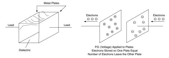
Fig. 17.28 A simple capacitor
