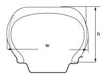
Fig. 1.1 Aspect ratio of a tyre (Example 1.26)
