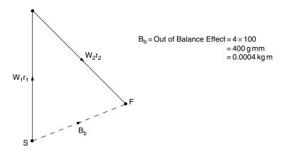
Fig. 12.5 Balancing diagram
