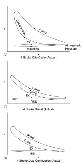
Fig. 15.5 Indicator diagram for (a) petrol engine; (b) lowspeed diesel engine; (c) high-speed diesel engine - dual combustion.
