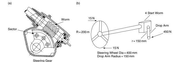
Fig. 8.8 Worm and sector steering gear (Example 8.12)
