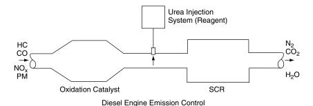
Fig. 16.7 Selective catalyst reduction (SCR) system
