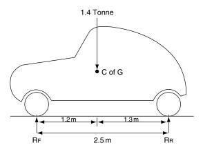
Fig. 7.9 Axle loadings (Example 7.6)
