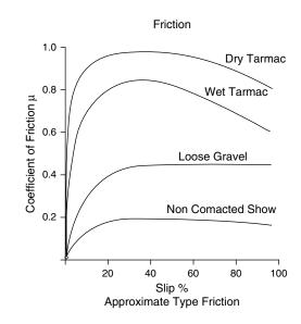
Fig. 9.9 Tyre friction
