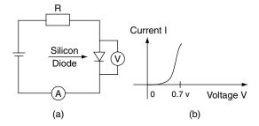
Fig. 18.4 Current-voltage in forward biased diode
