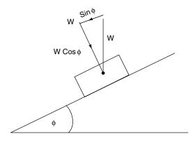
Force Down Slope to Move Block Against Friction = W  $\sin \phi$  Force Pressing Block on to Slope = W  $\cos \phi$
