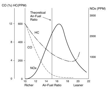
Fig. 16.3 Relationship between air-fuel ratio and exhaust emissions
