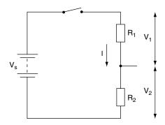
Fig. 18.14 The voltage divider
