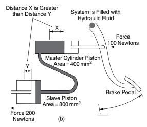
Fig. 5.10 Hydraulic brakes and pressure
