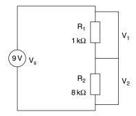
Fig. 18.15 Example - voltage divider
