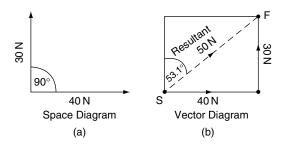
Fig. 5.3 Vector diagram - adding forces
