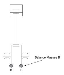
Fig. 12.11 Single-cylinder balance masses
