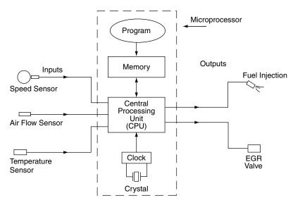
Fig. 18.1 Microprocessor-controlled vehicle systems
