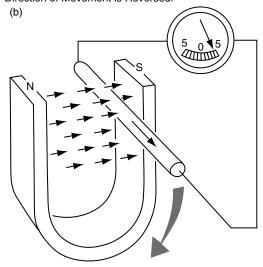
Fig. 17.20 Current flow, magnetic field and motion
