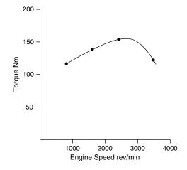
Fig. 14.8 Torque vs. engine speed
