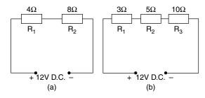
Fig. 17.7 Resistors in series
