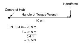
Fig. 7.11 Torque calculation (Example 7.7)
