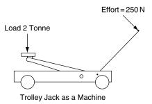
Fig. 8.6 Trolley jack (Example 8.9)
