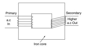
Fig. 17.26 Principle of the transformer
