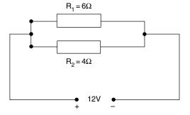
Fig. 17.8 Resistors in parallel
