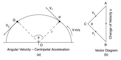
Fig. 10.5 Centripetal acceleration
