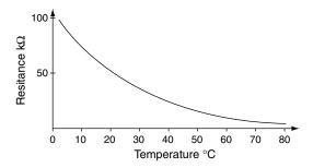
Fig. 18.5 Negative temperature coefficient
