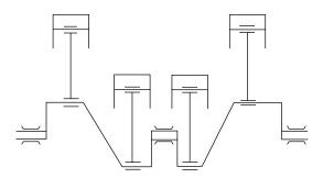
Fig. 12.12 Four-cylinder in-line engine
