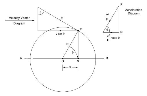
Fig. 12.14 Simple harmonic motion (SHM)
