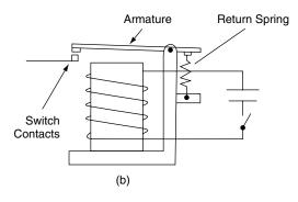
Fig. 17.19 (a) Magnetic field of a coil; (b) relay
