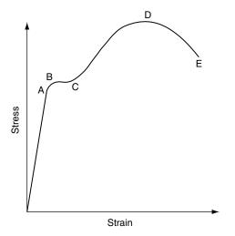
Fig. 6.3 Stress vs strain for a tensile test on a steel specimen
