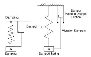
Fig. 12.18 Simple vibration damper
