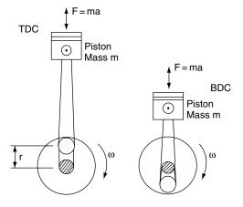
Fig. 12.7 Forces acting on reciprocating parts
