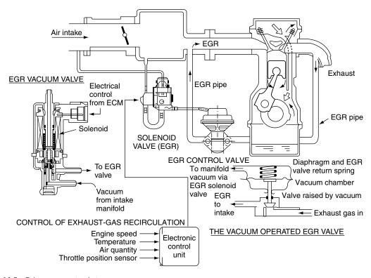
Fig. 16.5 Exhaust gas recirculation system
