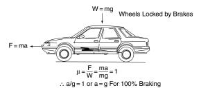
Fig. 9.10 Braking efficiency
