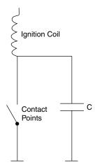
Fig. 17.30 Capacitor in contact breaker ignition circuit
