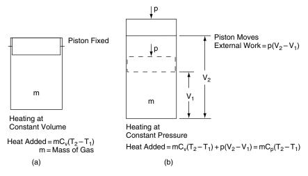
Fig. 13.1 Heating a gas at constant pressure and constant volume
