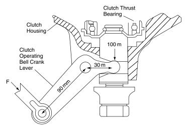
Fig. 7.16 Bell crank clutch mechanism (Exercise 7.1)
