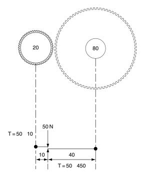
Fig. 7.13 Torque multiplication
