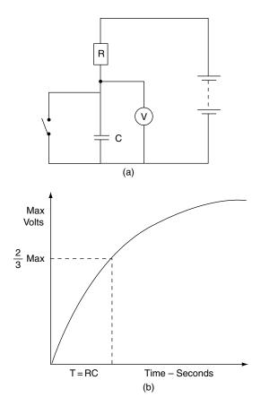
Fig. 17.29 Charging a capacitor
