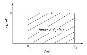
Fig. 13.2 Constant pressure expansion of a gas
