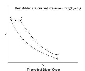
Fig. 15.3 pV diagram for the diesel cycle
