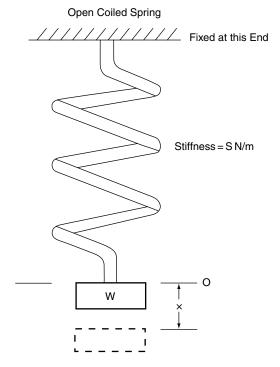
Fig. 12.15 SHM of open coiled spring
