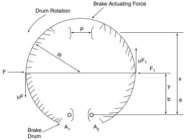
Drum Radius = R Actuating Force = P F and  $F_1$  = Normal Force Created by P  $\mu$ F and  $\mu$ F $_1$  = Friction Forces
