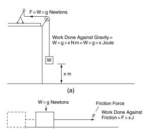
**Fig. 8.1** Work = force  $\times$  distance
