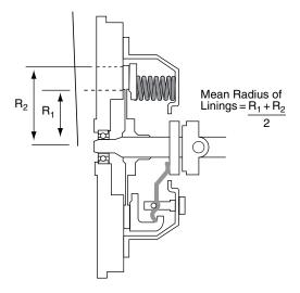
Fig. 9.3 Single plate clutch
