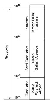
Fig. 17.2 Relative conductivity scale for various materials
