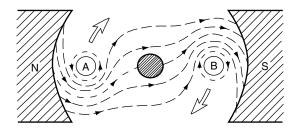
Fig. 17.22 Opposing magnetic fields – the motor effect
