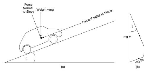
Fig. 11.6 Forces acting on vehicle on a gradient
