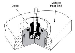
Fig. 18.12 A diode and its heat sink
