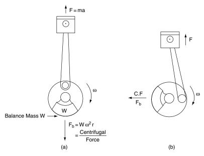
Fig. 12.8 Effect of balance weight (mass)
