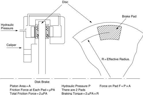
Fig. 9.8 Disc brake
