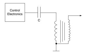
Fig. 17.31 A capacitive discharge ignition system
