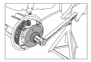
Fig. 7.10 Torque wrench
