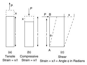
Fig. 6.8 The three types of strain
