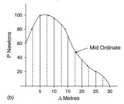
Fig. 8.4 Work diagram – variable force (Examples 8.4 and 8.5)
