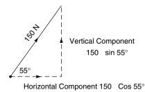
Fig. 5.7 Resolution of a force (Example 5.3)
