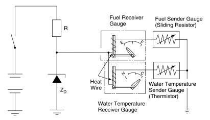
Fig. 18.6 The Zener diode as a voltage regulator
