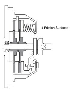
Fig. 9.4 Twin plate clutch (Example 9.2)
