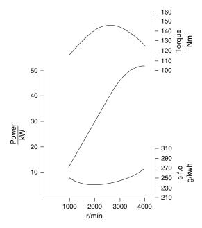
Fig. 14.11 Characteristic curves of diesel engine variables
