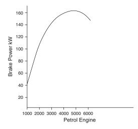
Fig. 14.6 Brake power vs. engine speed
