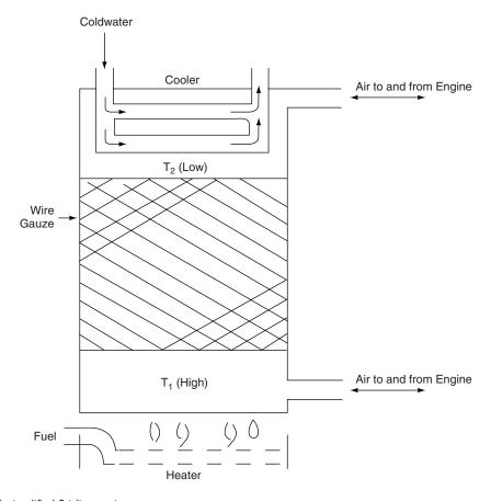
Fig. 15.6 A simplified Stirling engine regenerator
