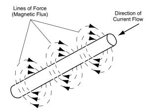
Fig. 17.16 Magnetic field of straight conductor
