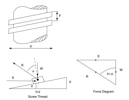
Fig. 9.14 Screw thread as inclined plane
