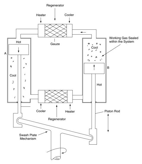
Fig. 15.7 Double-acting Stirling engine
