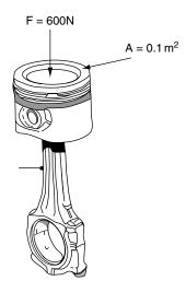
Fig. 3.1 Pressure in a cylinder
