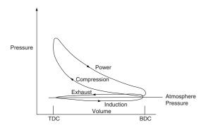
Fig. 14.3 Indicator diagram for a 4-stroke engine
