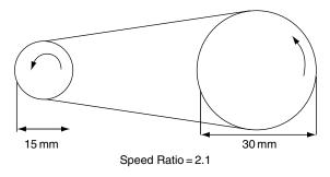
Fig. 9.6 Speed ratio - belt drive
