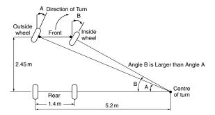
Fig. 4.21 Steered angles (Example 4.18)
