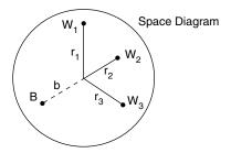
Fig. 12.3 Three unbalanced forces in the same plane
