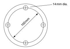
Fig. 6.6 Propeller shaft coupling flange (Example 6.4)
