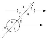
Corresponding, Angles are Equal A=H; B=E; C=F, D=G. Alternate Angles are Equal D=E; C=H.
