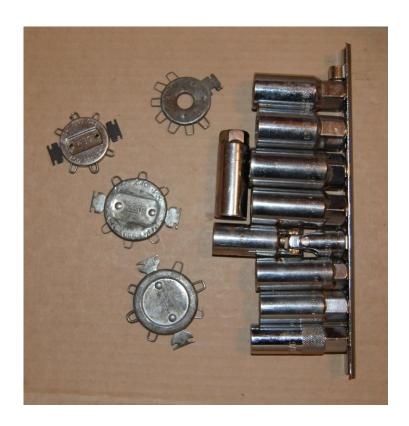
Spark plug gap tools and sockets.
