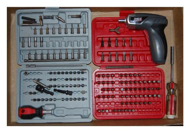
These are all the screwdriver bits I have been able to find so far. Flat, Phillips, Tri-wing, hex - SAE, metric, and tamper proof, Torx and Tamper-proof Torx, game system, and others. These are handy to have in addition to regular screwdrivers.
