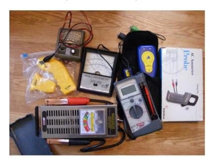
Multimeters, a battery tester, tach/dwell meter
