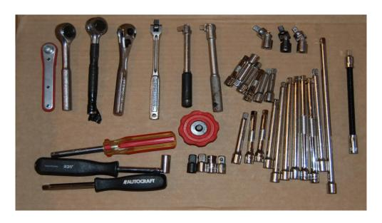
Top left: A 1/4" screwdriver bit ratchet, two cheap ratchets, a Craftsman ratchet, a Craftsman breaker bar, two cheap breaker bars.
