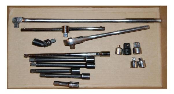
At the top is the large Craftsman breaker bar. Below that is a sliding t-handle from Tractor Supply. Then, a u-joint and Craftsman ratchet. Bottom left are extensions. To the right of those are: adapter to drive 1/4" sockets, 3/4" sockets, and 3/8" sockets.
