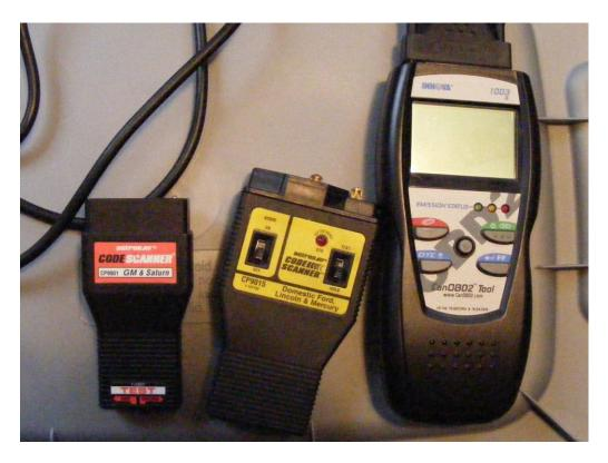
GM OBD 1 scanner, Ford OBD 1 scanner, and an OBD 2 scanner
