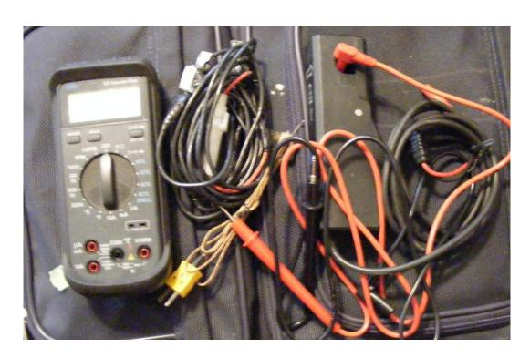
A meter with temperature and RPM leads.
