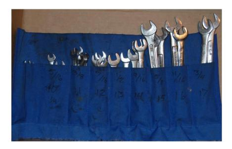
Combination wrenches. Get the best you can - two of each size to have one to hold a bolt still while you turn the nut with the other one. Deep-well sockets are faster, but sometimes, they don't fit.
