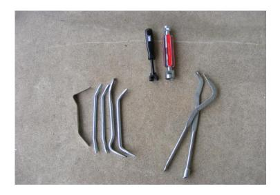
Lower left: Tools for turning adjusters on vehicles with drum brakes. Note that some vehicles are self-adjusting and do not use these.
