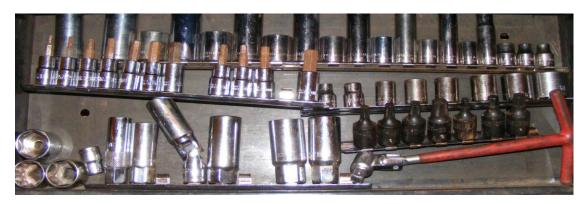
At the top are regular and deep well standard sockets. The slightly rusted sockets are SAE and metric hex bits. To the right of those, are SAE 12-point sockets. Below those are Torx sockets. I have a variety of brands, but the most commonly used sockets are name brand.
