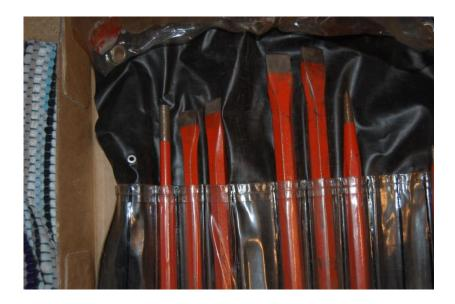
Pin punches for removing pins. Cold chisels for cutting metal. Tapered punches for aligning holes.
