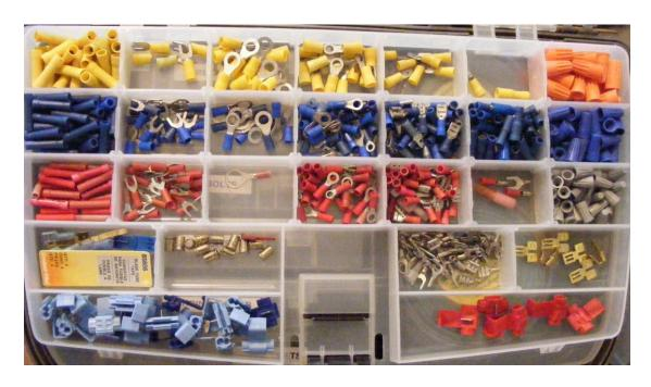
These are assorted wire terminals for different sizes of wires.
