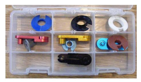
These are for newer fuel line, transmission and oil cooler lines.
