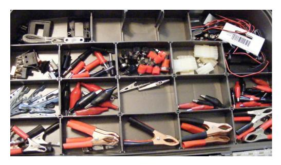
A variety of alligator clips, switches, jacks, and 9V battery leads.
