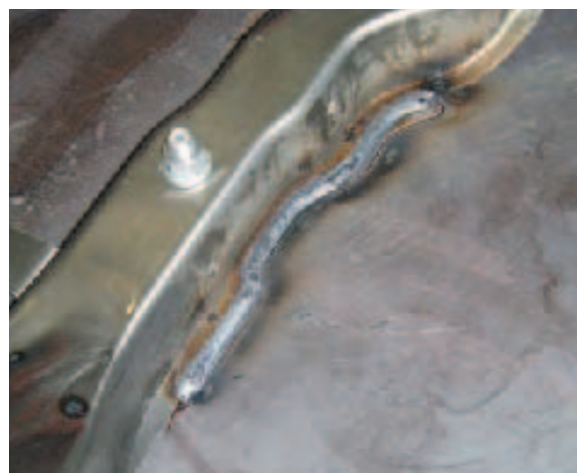
A very common joint; overlap. Plate thickness is 1.5mm and welding speed in this case 32 mm/sec.
