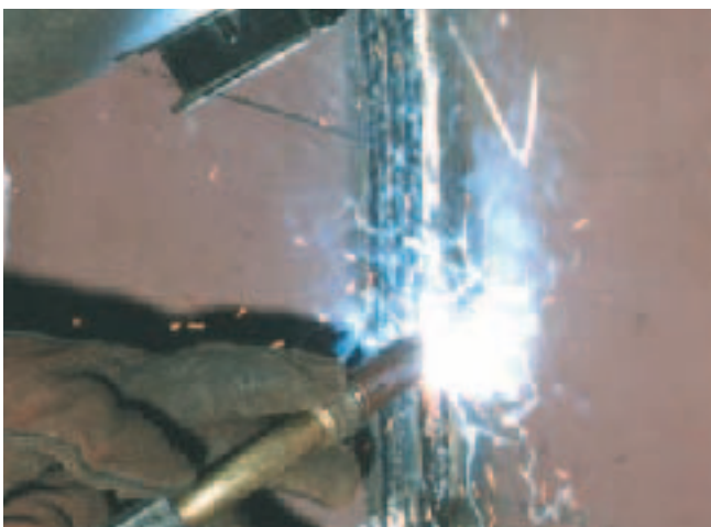
Figure 4. Vertically-up welding of a pedestal part.
