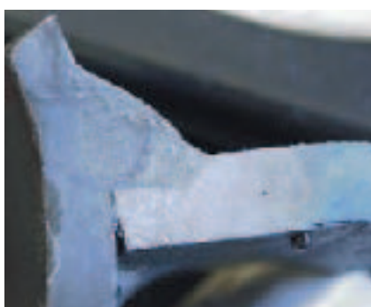
Figure 11. Etched cross-section A-A of a scaffolding component welded with PZ6105R.
