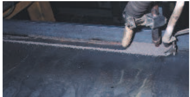
Figure 2. SAW with OK Tubrod 14.00S/OK Flux 10.71. Note that the slag is self releasing.
