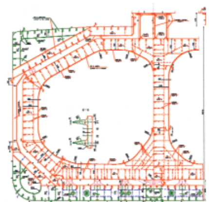
Figure 2. Cross-section of an LPG tank consisting of two independent compartments. The red lines are DNV NV 2-4 class steel and the green lines are standard shipbuilding quality.
