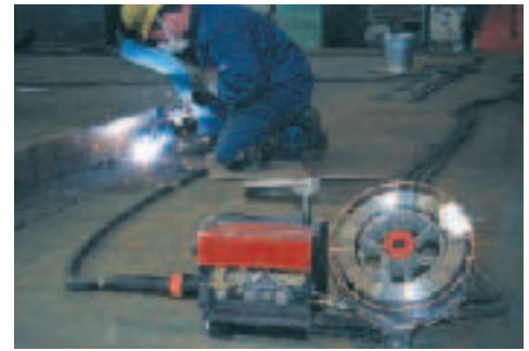
Figure 9. FCAW under CO 2 gas protection with PZ6116S.
