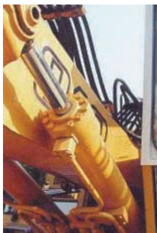
Figure 2. Lifting hydraulics for the boom.
