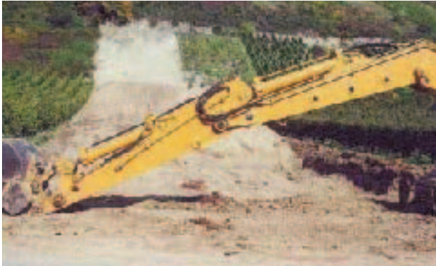
Figure 3. Hydraulic cylinder for moving the bucket and jib.
