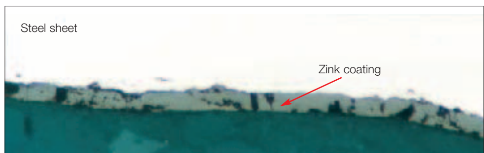
Figure 3. Transverse section through GMA-brazing seam on a body panel ( s = 0.8 \text{ mm} ). Location of section: underside of panel. A residual zinc coating is retained.
