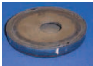
Figure 2. Safety component welded with PZ6105R
