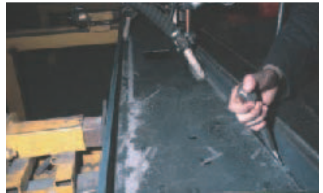
Figure 3. The self-released slag is easily removed.
