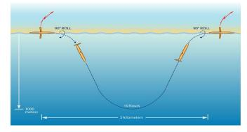
Buoyancy driven gliders can follow a saw-tooth pattern patter across ocean depth, periodically they transmit the data collected by onboard sensors to mother ship or shore by satellite communication. Gliders are extremely stealthy. They are quite, with very low self-noise, small acoustic cross section and leave a practically invisible wake.
