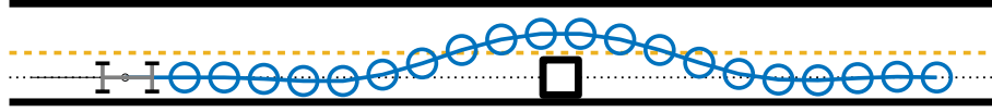
Figure 1.1: Example of motion planning around an obstacle. The centerline (dotted) is the reference trajectory, and the blue circles indicate the planned trajectory.
