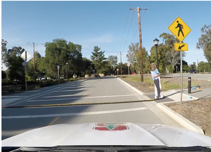
Figure 4.8: Experimental setup of pedestrian crosswalk using a cardboard cutout for the pedestrian that moves along a track. Depicts the pedestrian posture of stopped.
