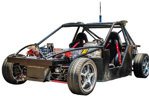
Figure 3.5: X1, an all electric, steer- and drive-by-wire research testbed.
