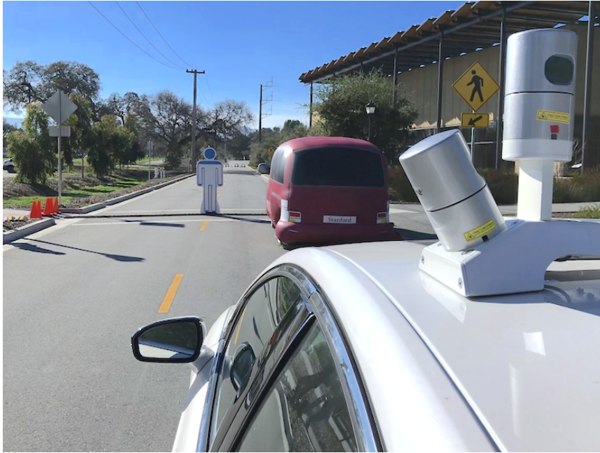
Figure 4.4: Experimental setup of occluded pedestrian crosswalk using an inflatable van for the occluding vehicle and a retro-reflective cardboard cutout for the pedestrian that moves along a track.
