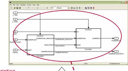
SWC description (e.g. ports, runnables) is exchanged via AUTOSAR XML
