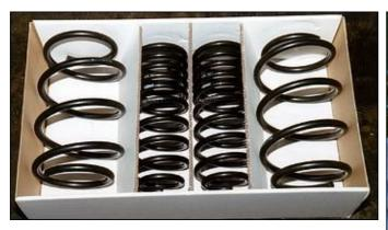
But, really, the Number One golden rule is a minimum of 100mm clearance between the road and the lowest point of the car. A sensible amount of lowering that leaves enough bump travel and shouldn't have the car leaving the road whenever it hits a bump.
