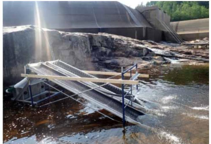
Figure 4: Example of an eel ladder style trap erected on the North Shore for the MFFP. Photo: Akian Gros-Louis Picard
