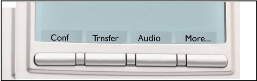
Figure 6: In-call context-sensitive soft keys lists the context-sensitive soft keys you can use to access menu items during an in-call session.
