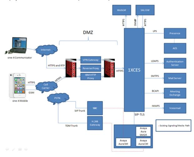
During installation, you can install Client Enablement Services with or without the Handset Server. The Handset Server facilitates the communication between the handsets and the Handset Services running in Client Enablement Services. Handset Services is a separate Java Application that you can install outside the Intranet, mostly in the DMZ. You can scale the Handset Server according to the number of Avaya one-X<sup>®</sup> Mobile users.
