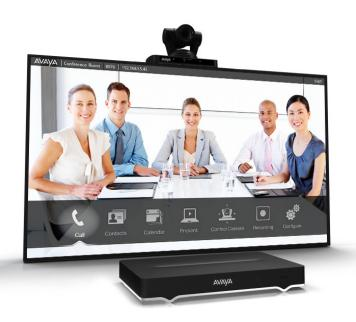
The Avaya Scopia® XT5000 is our flagship product in the Scopia series of room systems. The XT5000 incorporates dual 1080p/60fps live video and content, HD audio, simultaneous H.264 High Profile and Scalable Video Coding (SVC), and multi-party calling. The PTZ camera, supporting 1080p/60fps, offers 10x optical zoom (40x digital) and wide-angle capability for viewing details and an entire group.
