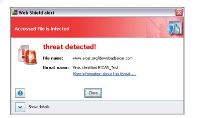
If AVG fails to identify the EICAR test file as a virus, you should check the program configuration again!
