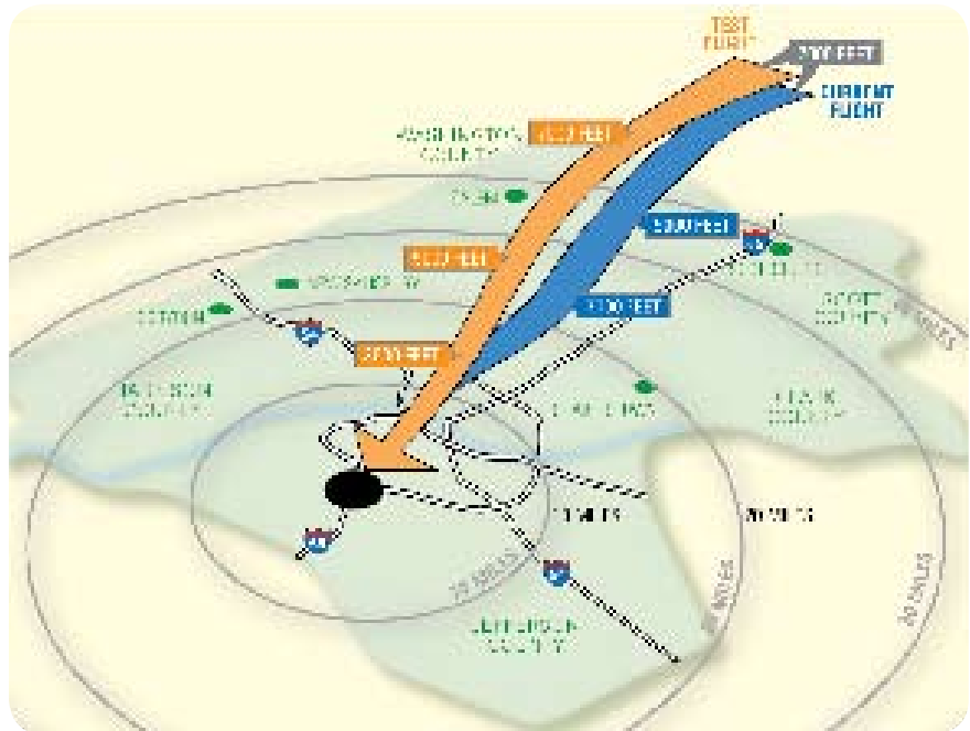
Standard flight paths, such as the one at Louisville (shown in blue) involve a series of stepped descents. New continuous descent approach procedures, collaboratively developed by an FAA/NASA/industry/academia team, have been shown reduce noise impacts by keeping aircraft higher, longer. They have also been shown to reduce fuel burn and emissions of local air quality pollutants. (Illustration © The [Louisville] Courier Journal.)
