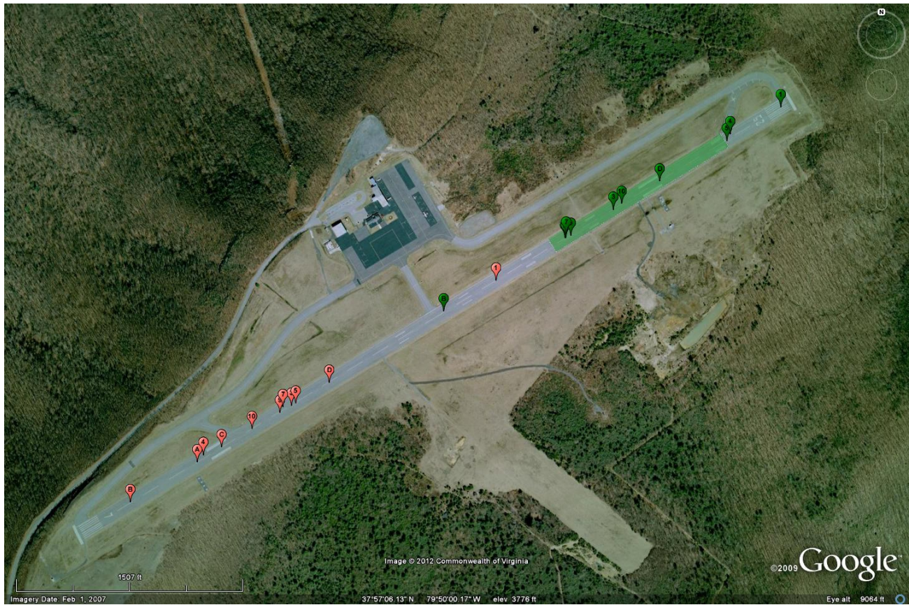
Figure 13. Touchdown zone (green rectangle) along with initial (green) and projected final (red) landing points
