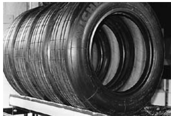
Tires should be stored vertically in racks
