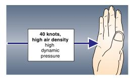
Figure 1-14 Dynamic pressure is greater in dense air.
