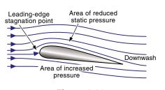
Figure 1-12 Pressure around an airfoil.
