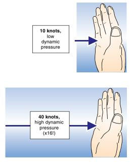
Figure 1-13 Dynamic pressure increases with airspeed.
