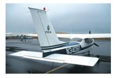
Figure 1-7 Vertical stabilizer and rudder.
