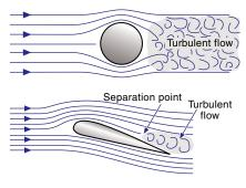
Figure 1-10 Turbulent flow.
