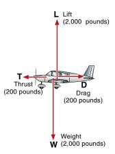
Figure 1-3 The four main forces are in equilibrium during unaccelerated flight.
