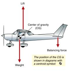
Figure 1-4 Weight acts downward through the center of gravity (CG).
