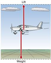
Figure 1-2 The airplane is supported by the ground, and in the air by lift.
