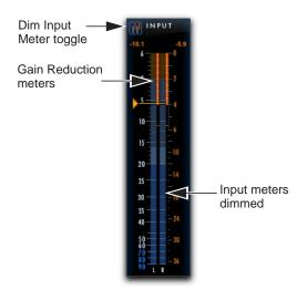
Gain Reduction meters shown with Input meters dimmed
