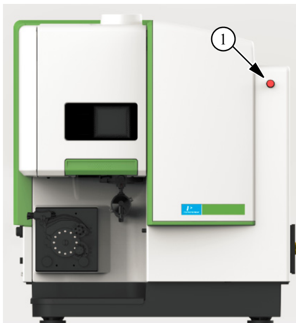
Figure 3-9 Location of Red Emergency Plasma Off Switch .
