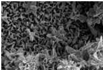
Scanning Electron Microscope image of HydroSet material crystalline microstructure at 15000x magnification
