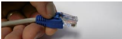
Pull boot back to access lock clip
