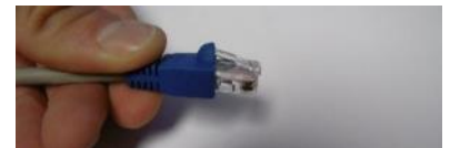
Slide boot back over lock clip
