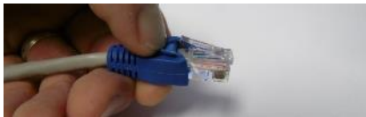
Pull boot back to access lock clip
