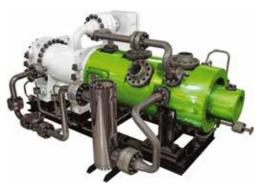
**Overhung Single Stage** – Overhung compressors are mainly used as boosters in petrochemical applications or for recycle in polypropylene and polyethylene plants. The single-stage overhung configuration is simple and easy to maintain. Almost all gases can be handled by this type of compressor with appropriate construction materials and seal systems.
