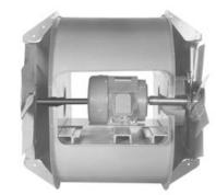
Single stage and two stage bifurcators are available in a wide range of sizes and air movement capacities. Direct drive models are available with propeller diameters from 12" to 60" and air capacities of 750 to 80,000 CFM. Belt drive single stage bifurcators are available on special order. Our engineering department will work with any customer to satisfy needs for belt drive bifurcators.
