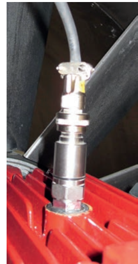
Sensor position on motor center (A1: VTV 122)
