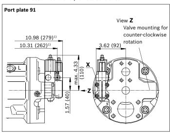
**▼** DRG - Pressure controller, remote controlled
