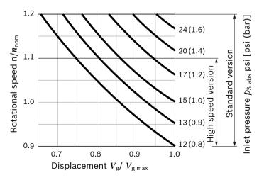
During continuous operation in overspeed over  $n_{\text{nom}}$ , a reduction in operational service life is to be expected due to cavitation erosion.
