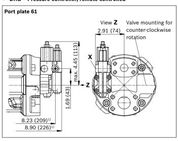
**▼** DRG - Pressure controller, remote controlled
