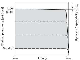
Characteristic curve valid at  $n_1$  = 1500 rpm and  $\theta_{fluid}$  = 120 °F (50 °C).
