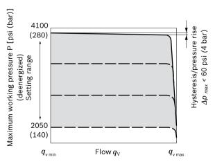
Characteristic curves valid at  $n_1$  = 1500 rpm and  $t_{fluid}$  = 122 °F (50 °C).
