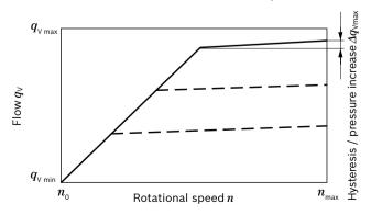
Characteristic curve valid at  $n_1$  = 1500 rpm and  $\theta_{fluid}$  = 120 °F (50 °C).
