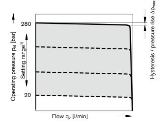
In order to prevent damage to the pump and the system, this setting range is the permissible setting range and must not be exceeded.
