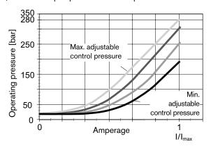
Hysteresis of the static current-pressure characteristic < 3 bar Influence of pressure setting on stand-by  $\pm 2$  bar
