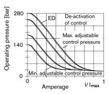
Hysteresis of the static current-pressure characteristic < 3 bar
