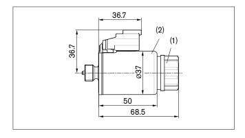
Before finalizing your design request a certified installation drawing. Dimensions in mm.
