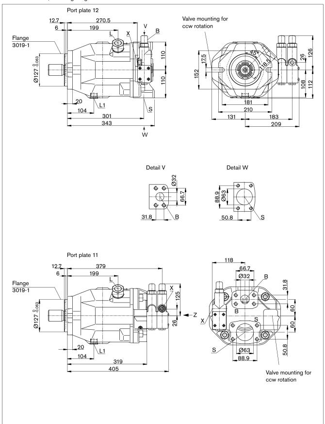
Before finalizing your design request a certified installation drawing. Dimensions in mm.
