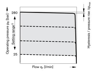
In order to prevent damage to the pump and the system, this setting range is the permissible setting range and must not be exceeded.
