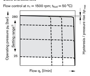
1) In order to prevent damage to the pump and the system, this setting range is the permissible setting range and must not be exceeded.
