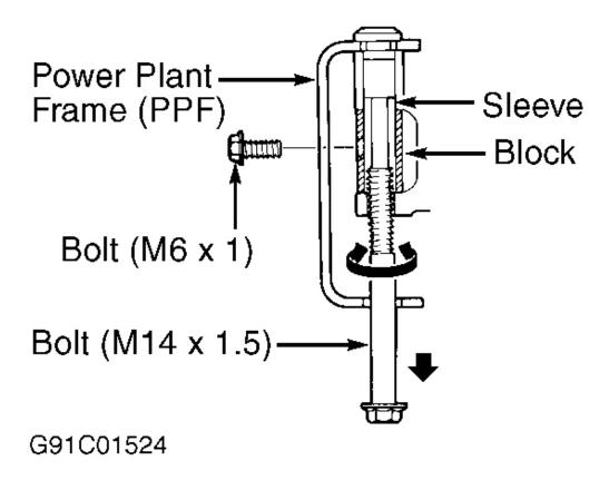
Fig. 7: Removing Reamer Bolt Sleeve (Miata) Courtesy of MAZDA MOTORS CORP.
