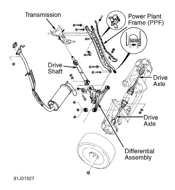
Fig. 5: Exploded View of Differential Components (Miata) Courtesy of MAZDA MOTORS CORP.
