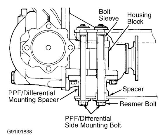
Fig. 6: View of Power Plant Frame Components (Miata) Courtesy of MAZDA MOTORS CORP.
