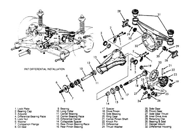
Fig. 4: Exploded View of Differential Assembly (RX7) Courtesy of MAZDA MOTORS CORP.
