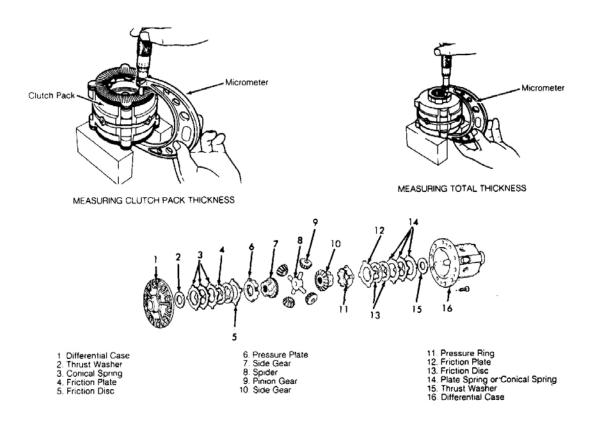
Fig. 9: View of Limited Slip Differential (LSD) Assembly (RX7) Courtesy of MAZDA MOTORS CORP.
