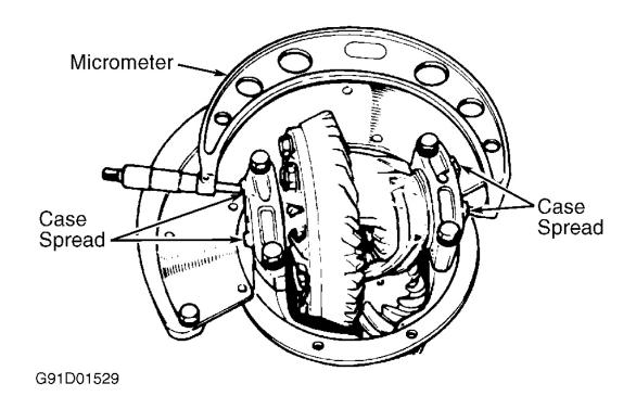
Fig. 12: Measuring Carrier Case Spread Courtesy of MAZDA MOTORS CORP.
