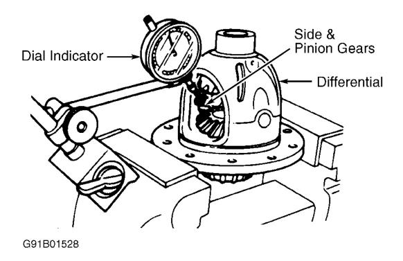
Fig. 10: Measuring Carrier Gear Backlash Courtesy of MAZDA MOTORS CORP.
