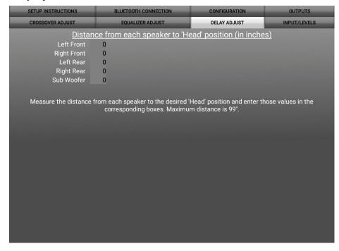
Allows a delay of each channel, up to 10 milliseconds. First measure
