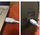
Connect the A-to-A USB cable to both the system USB and the computer. On the Axygen system, ensure the USB is plugged into the lower USB on the right hand side of the instrument.
