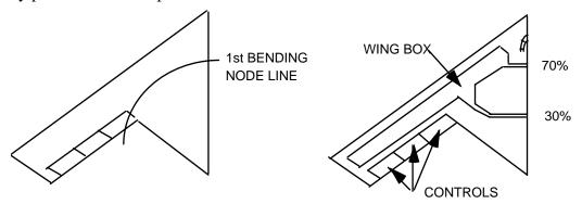
Figure 3-7. Structural Bending of the Wing at First Bending
