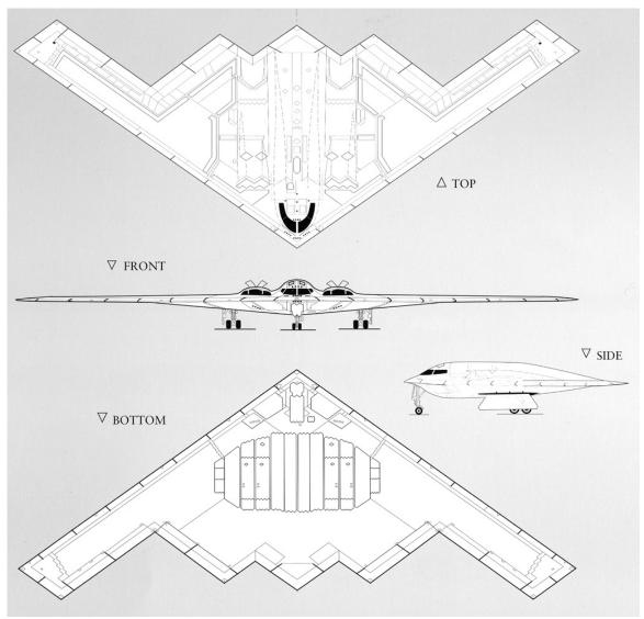
Figure 2-1. External View Drawings of the B-2 Aircraft [1]
