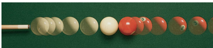
FIGURE 7-14 In this multiframe photo of a head-on collision between two balls of equal mass, the white cue ball is accelerated from rest by the cue stick and then strikes the red ball, initially at rest. The white ball stops in its tracks, and the (equal-mass) red ball moves off with the same speed as the white ball had before the collision. See Example 7-7, part (b).
