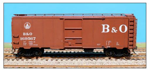
Now to the shot that many of you were waiting for, the B&O model with the Deco end. This car is painted the box car brown favored by C&O/B&O at the time. It is not the same color as the C&O model. Note that, as on the prototype B&O cars, the tack board and routing card board are in different places on the box car door.
