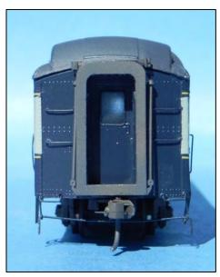
Detailing differs between the two ends; the brakewheel is on the kitchen end.
