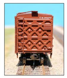
This is the end that launched a thousand models. IM did an excellent job of recreating this classic box car part. Missing however, is the plate that held the mounting for the coupler lift lever. See the grounded box car on the previous page, which still has this part and the lever.
