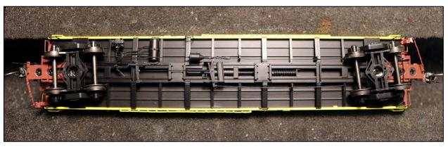
The detail on the underbody of the B&O model made me gasp. Note the wonderful rendering of the Keystone cushioning as well as the brake piping. One impressive detail is the rubber hose connected to the ABD valve. Sliding sill cars needed a flexible connection in this spot. Most model makers ignore this detail, but not Moloco.
