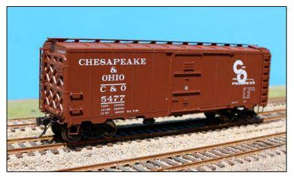
Intermountain's nice model of C&O 5477 shows the striking end and the 3-panel Creco door. This model is in the post-war "For Progress" lettering scheme. At least some C&O cars eventually got futura demi-bold lettering instead of the Roman used here. Still others would have been refurbished and repainted for the B&O.
