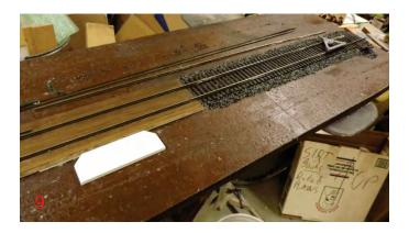
**Photo 9** Spiking the approach rails to the scale is the next operation. The white foam core piece is for a 1906 16' 6" x 6' B&O scale house foundation. Spiking was done to fine scale standards. Spikes were driven in the "A" pattern on two ties at the scale pit end and two ties at the switch end. The "A" pattern uses two spikes per tie plate driven diagonally opposite each other to hold the rail. A long straight edge was used to hold the rail in alignment while spiking.
