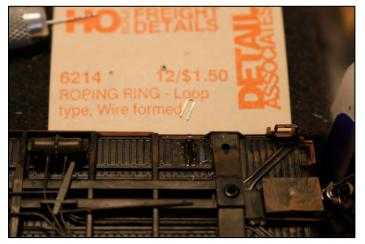
The author used a pin vise with a #76 bit to drill two small holes in the car floor and install Details Associates #6214 roping loops. He cemented them into place with thick ACC. The shiny spot left by slopped over glue was retouched with dull paint later.
