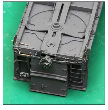
little before separating. I brushed a thin layer of Grimy Black paint on the magnet... enough to reduce its magnetism to prevent dragging a car during uncoupling.
