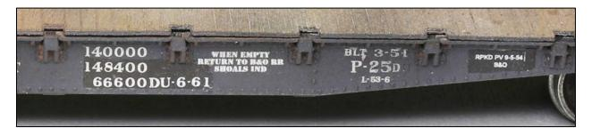
After decals were set and dried, I replaced all steps with Tichy 3038's and a few grab irons that had broken or I found were improperly located by the manufacturer with .010" phosphor bronze wire bent to shape and CA'd in place. Each step was pinned to the car with a .010" wire because glue alone was not strong enough.
