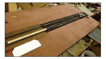
**Photo 5** Stained timbers for the scale's rails have been glued to the bottom supports and the 'I' beams mounted to the underside of the deck, following the drawing. Rails for the scale bed have been cut to length. Eighteen doubled <sup>1</sup>/<sub>4</sub>" styrene 'I' beams were cut to length and cemented at marked-off centers on the underside of the wood decking, following the prototype drawing.
