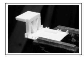
2 Add the short brace as shown. It will be necessary to file it to fit. Note that it fits against the raised part of the Base Mount. Do Both Sides.
