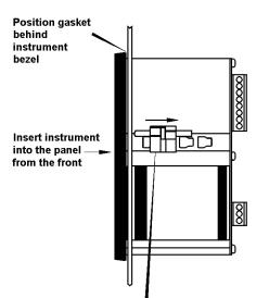
Slide panel mounting clip into the slotted rail on the side of the enclosure. Four clips are required to achieve an IP66 seal between instrument and panel.
