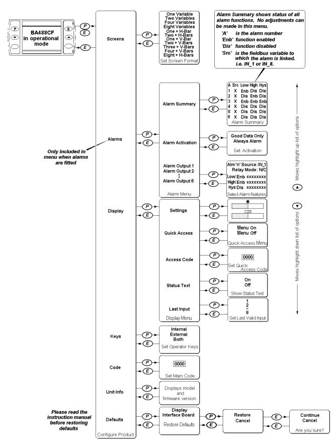
Fig 7 Structure of Configuration Menu
