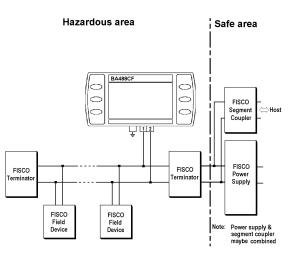
Fig 2 FISCO fieldbus system
