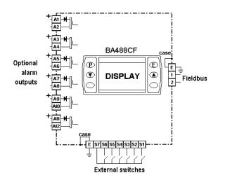
Fig 1 Simplified block diagram of BA488CF-F
