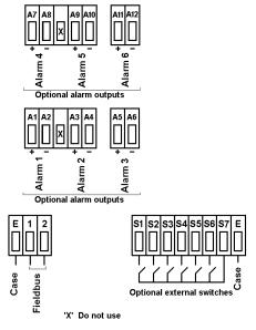
Fig 6 Installation and terminal connections
