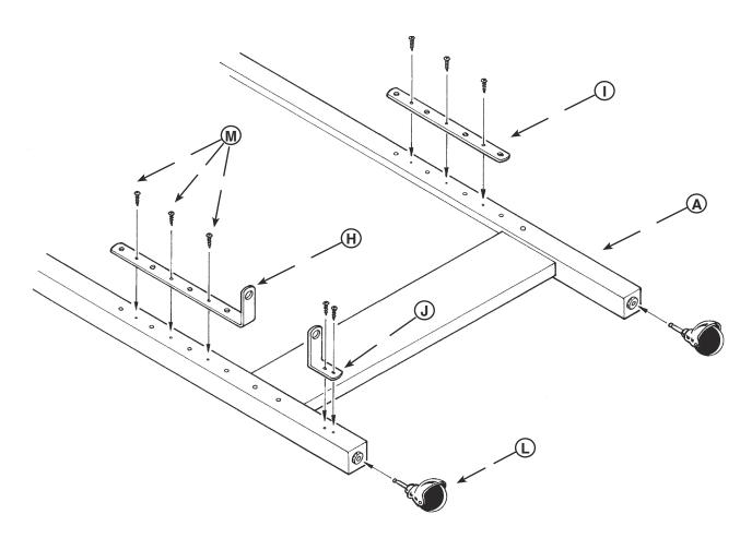
Attach the Front Bracket (H), the Back
