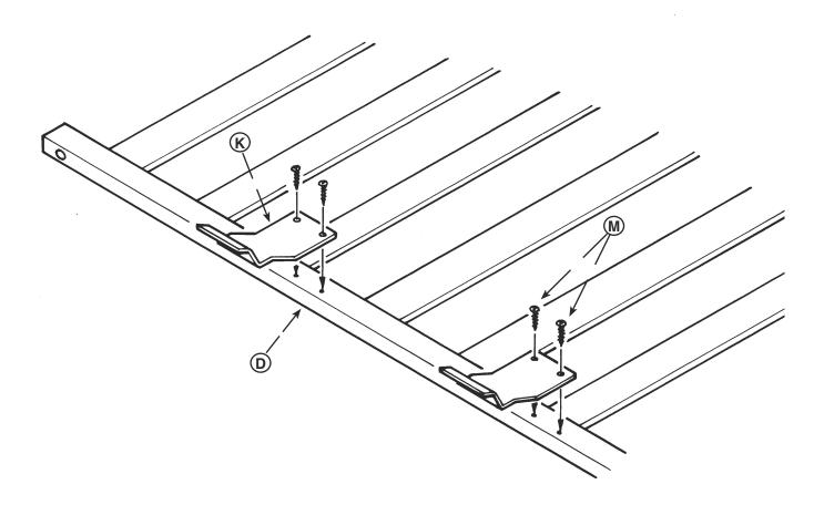
Attach the 2 Strike Plates (K) to the front gate using 4 of the Wood Screws (M). Note, the pilot holes are pre-drilled.
