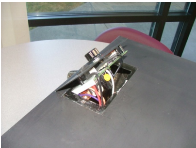
Insert wires and tilt controller
