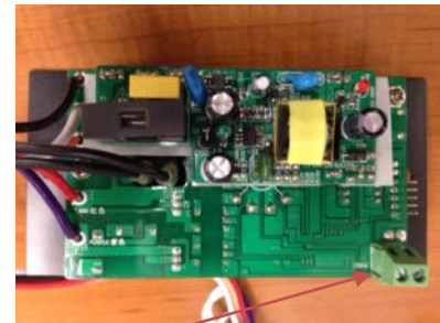
Install RTD wires to connector.
