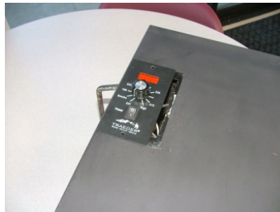
Set controller flat and insert fuse from behind.
