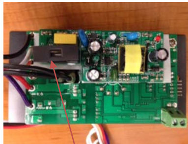
remove fuse cap and fuse
