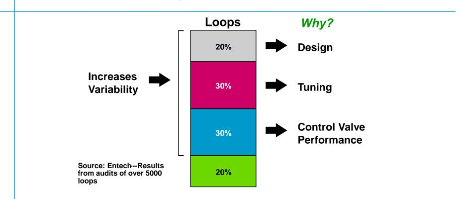
The undesirable behavior of control valves is the biggest contributor to poor loop performance and the destabilization of product uniformity".
