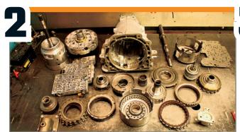
All the pieces of the puzzle are laid out to ensure no mistakes are made during the assembly process. The assembly of any automatic transmission can be compared to the most complicated layer cake you have ever seen. It's like trying to stuff 10 pounds of sugar in a 5-pound bag. I assure you, all those pieces do fit in the 4L60E case.
