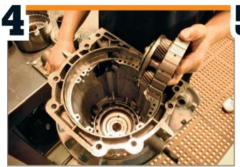
After all the parts are cleaned, the assembly begins with the installation of the rear gear and planetary gear into the bottom of the case. The 4L60E transmission consists of two complete planetary systems, which are responsible for all four forward gear ratios and the reverse gear.
