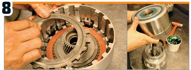
The input and reverse drums can then be assembled. These each receive a clutch pack and locking rings, and a sun gear is installed in the input drum. Once assembled, the drums are locked into place and installed in the case.
