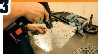
Here, larger holes are drilled in the valvebody plate to allow for a better flow of fluid across the valvebody. One thing we don't want to do is starve the system of fluid while trying to change gears. Orifice size can dramatically change shifting characteristics, and Level 10 knows exactly which ones to change per the application.
