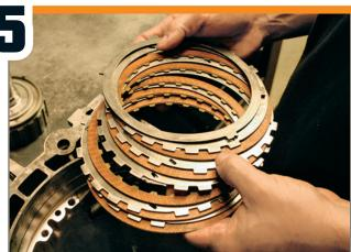
Next, one of three clutch packs is assembled in alternating layers of steel plates and clutch bands. The intricate system of fluid flowing through the valvebody directs fluid to one of these sets of bands, causing them to compress and engage the next gear.
