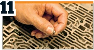
The case is then flipped over so we can continue work on the underside of the transmission. The valvebody balls are installed with grease to ensure they do not move during the process. These balls regulate the flow of fluid through the veins of the transmission and into the main case.
