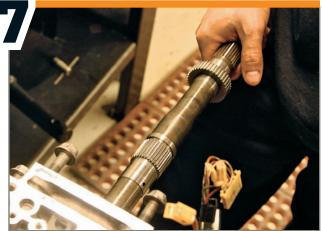
Next, the mainshaft is installed through the tail of the case. Once installed, the driveshaft will bolt up to the back of the mainshaft and the torque converter to the front. The mainshaft also works as a rotational center for all the moving parts inside the transmission.
