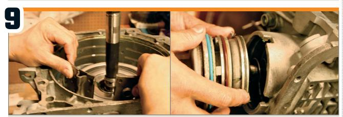
The intermediate band is installed next. Transmission fluid is guided through the valvebody and actuates the band, locking that part of the gears. In our electronically controlled transmission, the intermediate servo is activated via the automobile's ECM, and controls the action of the band. Level 10 assembles its own servos using a spring chosen per application, and a rubber seal to ensure no fluid is pushed through.
