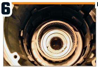
After installing the thrust washer, sun gear, and sun shell, the forward ring gear and forward planetary are installed. The planetary gears are at the heart of any automatic transmission. Each of the three components of the planetary can be held stationary, creating a different gear
