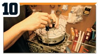
The PTS Super Pump is then installed, providing cooler transmission temperatures, lockup valve technology, increased pressure, and overall longevity. The stock pump can only pump so much fluid at a given time and is unsatisfactory for our application.
