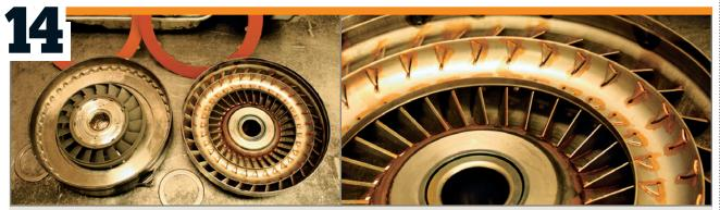
Level 10 also builds custom torque converters per application. Small changes in the angle and clearance of the veins in each of the components will affect stall speed, flash, and slippage. To keep things simple, we can say that the torque converter replaces the clutch in a manual transmission setup and transfers power from the engine to the transmission. In our case, we have yet to determine vehicle weight and rear gear ratio. Once we provide that information, Level 10 will create a custom
