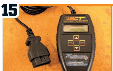
Level 10 utilizes this SCT Xcalibrator handheld tuner to set shift points, line pressure, and all the necessary information the ECM needs once the transmission is in the vehicle. Level 10 can also perform laptop tuning once the transmission is dropped in the vehicle. It provides full-service diagnostics and tuning after the purchase of a trans.
