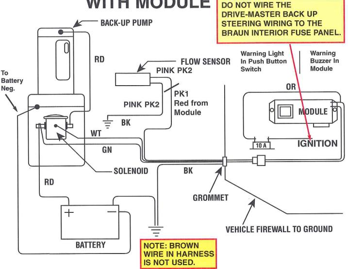
**WARNING:** THE IGNITION WIRE TO THE BACK-UP STEERING SYSTEM MUST BE A TRUE IGNITION WIRE. IF YOU ATTACH IGNITION WIRE TO AN ACCESSORY CIRCUIT THE BACK-UP STEERING WILL ACTIVATE WHEN YOU TURN THE VEHICLE OFF.
