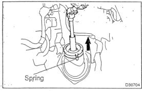
(b) Release the 3 springs and separate the dust cover.
