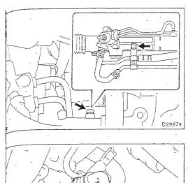
(c) Remove the bolt and separate the tube clamp.
