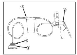
CAUTION: Do not run the engine while vacuum is applied to the power steering system. Damage to the power steering pump can occur.
