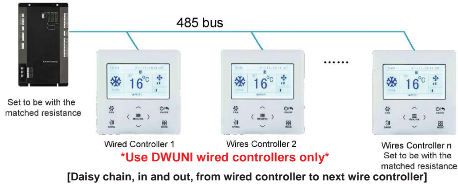
Fig. 5-9. Internet location and the matched resistance setting for single-split and multi-split units
