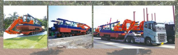
Self Loading-Unloding - using hydraulic spuds
