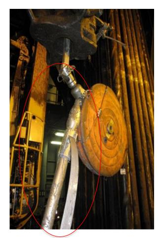
Wireline tool - 70kg @ 30m from drill floor
