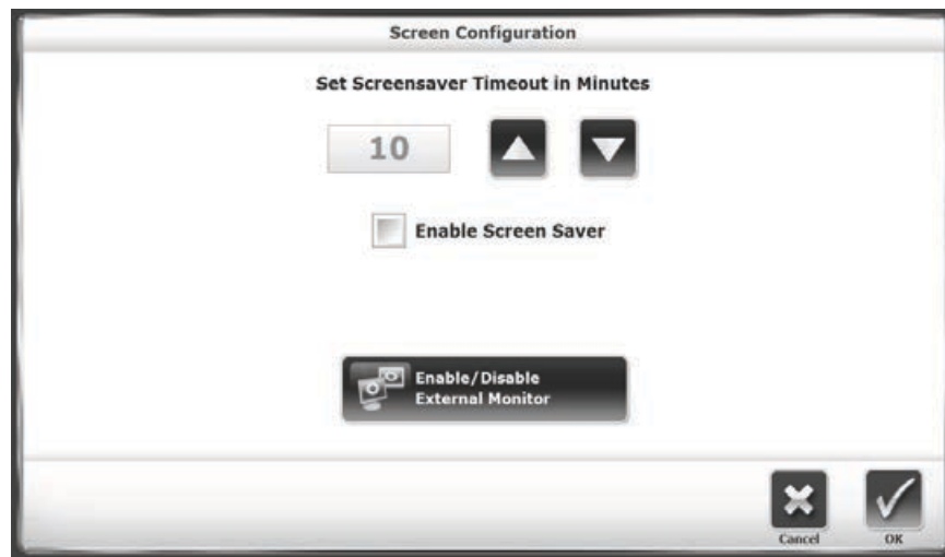
Figure 8.23. Screen Configuration settings, including the Screen Saver function (touch box next to Enable Screen Saver to activate), and the Enable/Disable External Monitor button.
