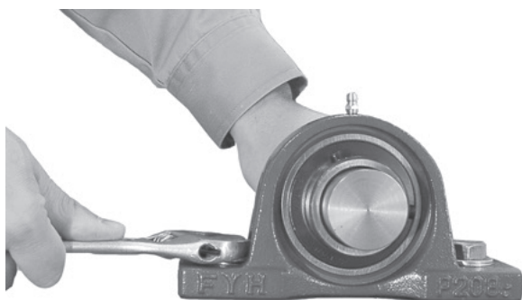
Fig. 14.4 Installation of setscrew units
