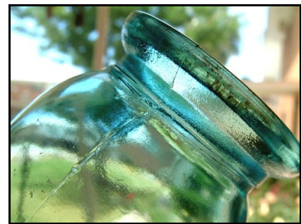
Figure 20 – Machine seams on wax-sealer finish
