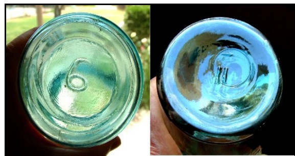
Figure 21 – Machine scars on wax sealer bases
