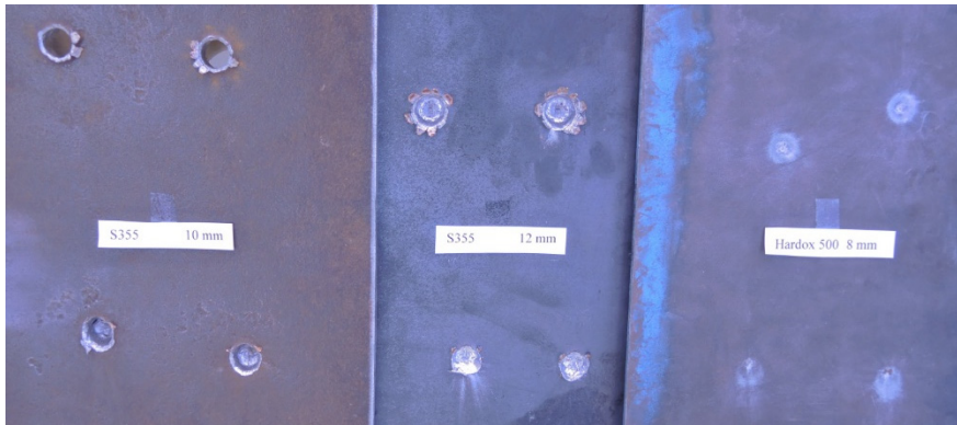
Figure 4: Results of experiment – impacts at the angle of 90^\circ are at the top of the plates, and those at 45^\circ at the bottom.
